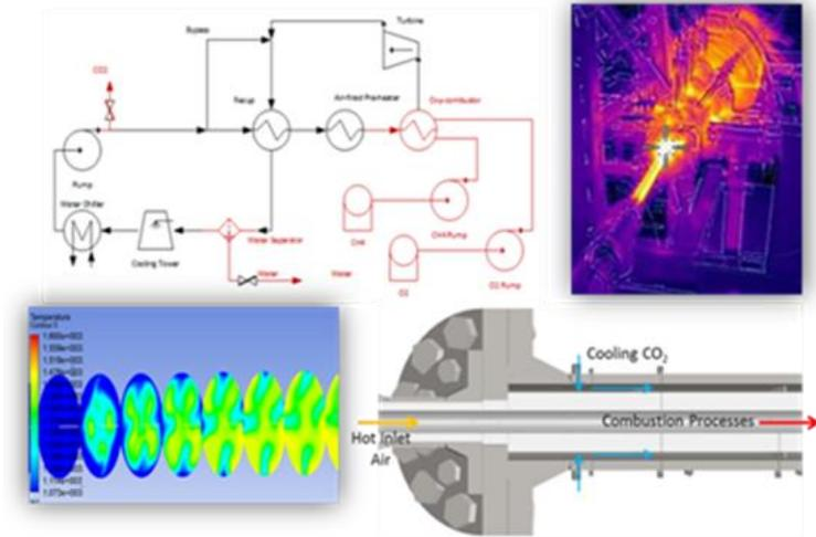
Direct Fired Supercritical CO<sub>2</sub> Oxy-Combustion: Bench Scale Testing and 1MW Scale Concept
