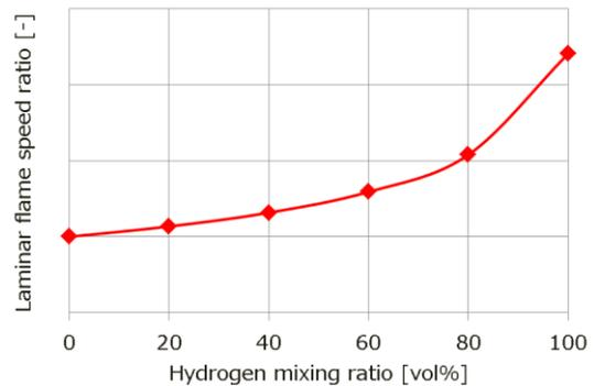
Fig. 4 Laminar flame speed with natural gas and hydrogen
