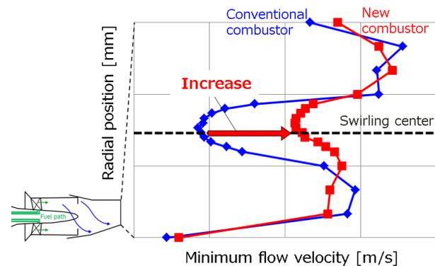
Fig. 8 Comparison of flow velocity distributions in swirling region
