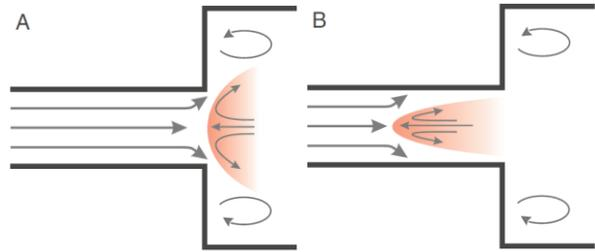
Fig. 3 Sketches of a stable flame(A) and a flame with flashback(B)
