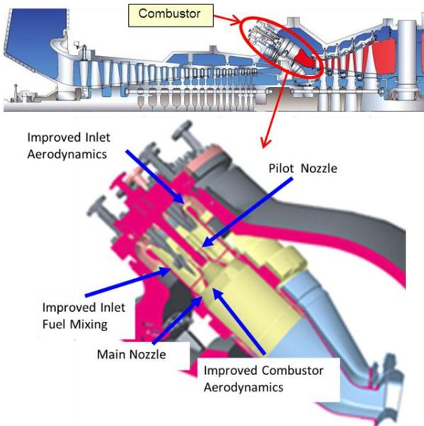
Fig. 5 Schematic of MHPS gas turbine DLN combustor
