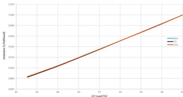
Figure 11 GT emissions vs power output
