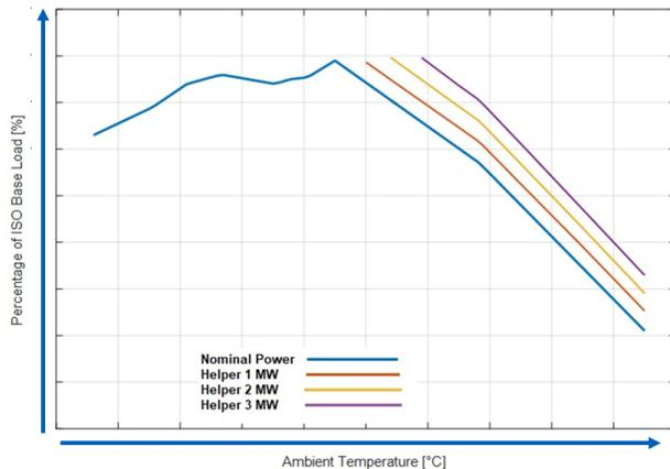
Figure 4 GT Power Output vs Ambient Temperature
