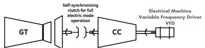
Figure 9 LP shaft hybrid configuration
