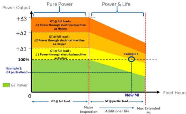
Figure 2 Power augmentation and life extension synergy
