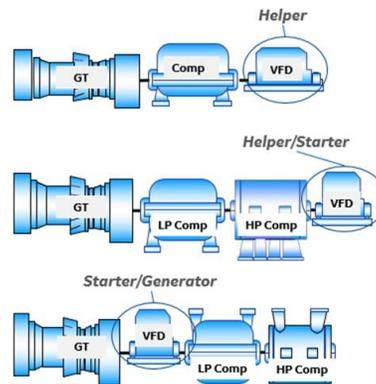
Figure 3 Layout options when VFD is used in LNG refrigeration GT driven trains
