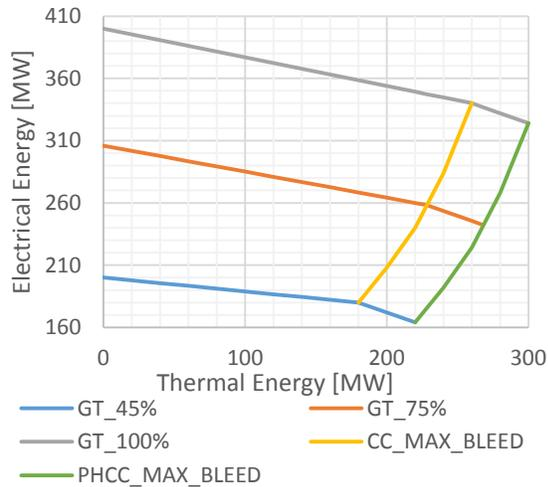
Figure 3 – PHCC in cogenerative configuration: a) Operational range and b) Performance
