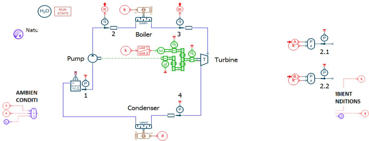
Figure 5 – Simcenter Amesim model of the simplified power plant steam cycle
