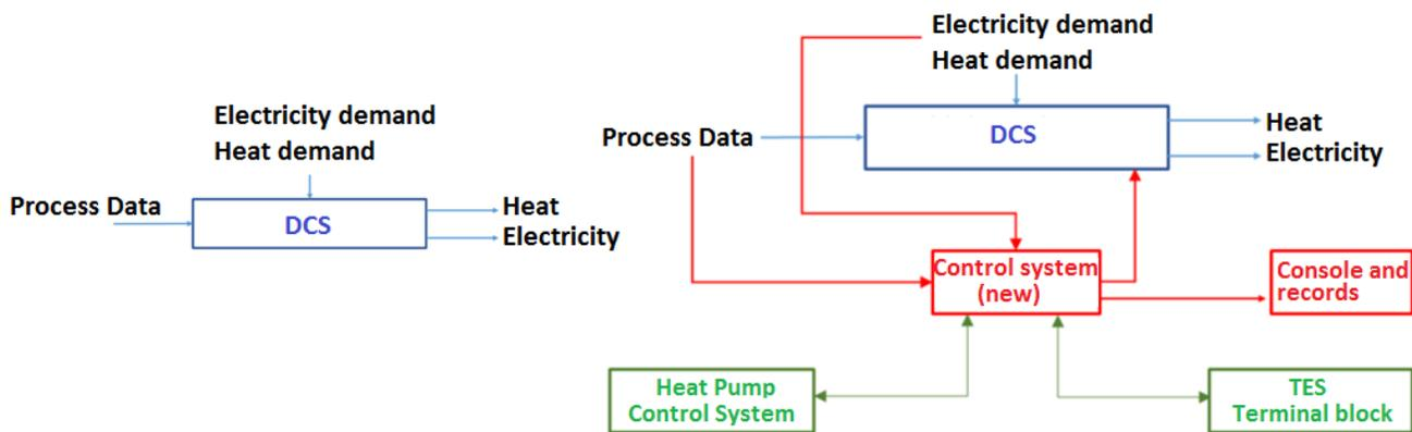
Figure 7 – Scheme of control scheme (a) as it is right now and (b) how it will be enriched within PUMP-HEAT
