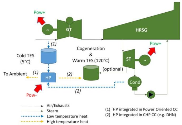
Figure 1 – Scheme of PHCC in PO (path 1) and cogenerative (path 2) configuration
