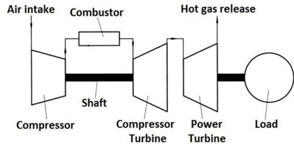
Figure 6. Twin-shaft industrial gas turbine
