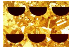
Micrograph of PCHE section [Southall, 2008]
