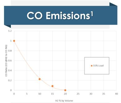
H<sub>2</sub> caused more complete combustion, reducing CO emissions
