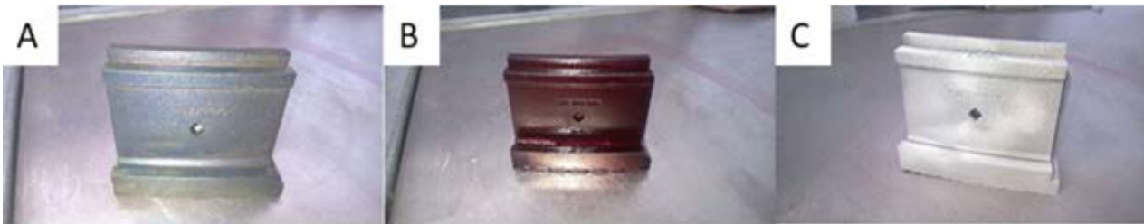
Figure 13: PT test being carried out on a shield (A) shows shield before inspection (B) shows the shield with contrast penetrant (C) shows the shield with the developer.
