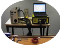
On-line measurement of organics (MEA, NH 3 , aldehydes...) and inorganics (NH 3 , CO 2 , H 2 O, NO x , CO ...) at ppm level
