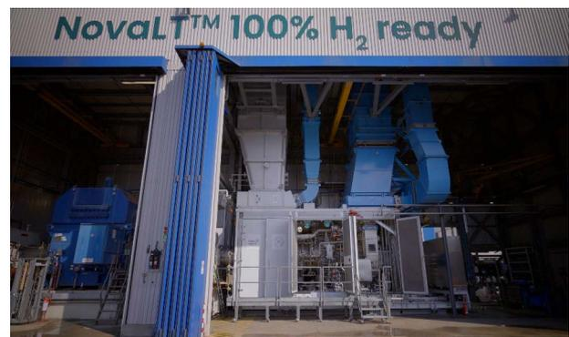
Figure 17 – NovaLT™16 100% hydrogen-ready gas turbine, installed on the Baker Hughes test bench at its Florence site (IT). Image courtesy of Baker Hughes.\*
