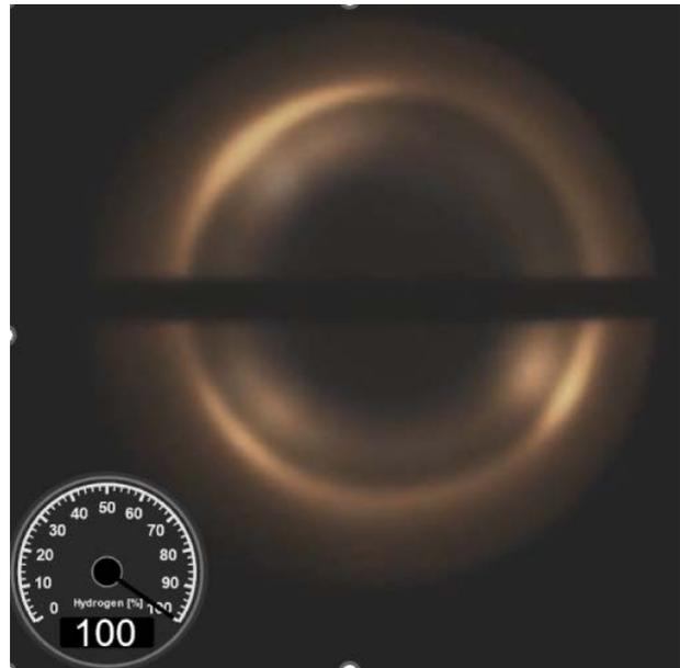
Figure 21 – FlameSheet™ combustor operating at 100% H<sub>2</sub>.
