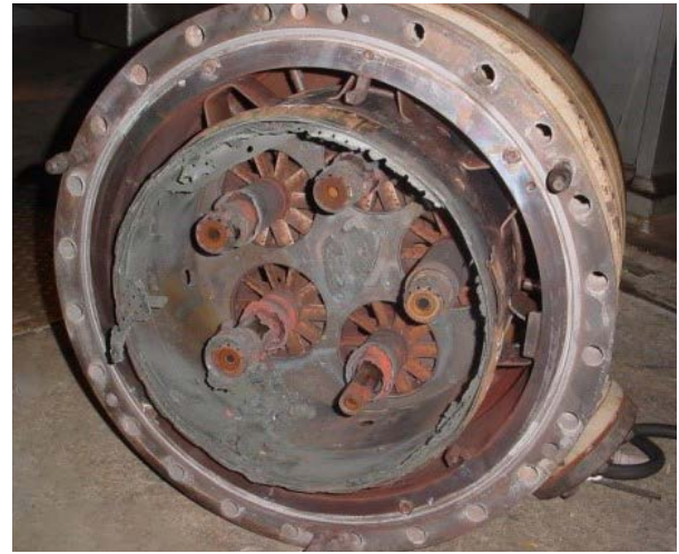
Figure 7 – Combustor damage due to high-frequency (2350 Hz) thermoacoustic instabilities due to inappropriate tuning of the machine [25].
