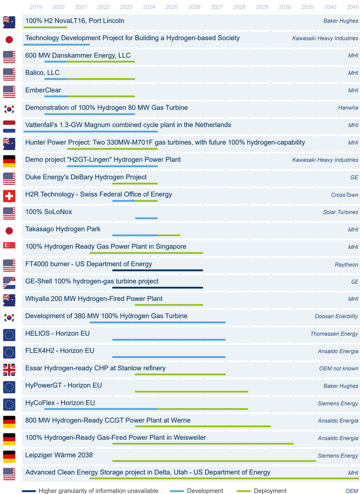
Figure 11 – Selected hydrogen gas turbine development and deployment projects listed by expected delivery timeline, country/region, and gas turbine OEM. Note each project includes a link for more details.
