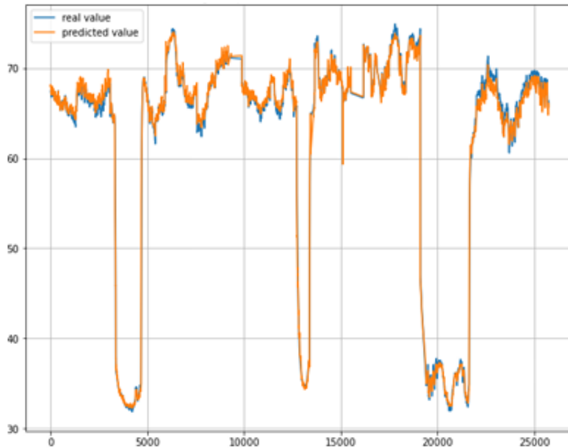
Actual and predicted values for the bearing temperature using Year 1 data as training data.
