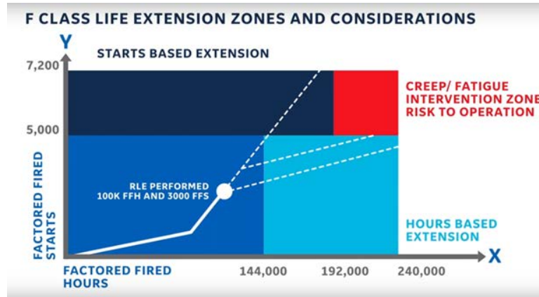
Figure 5: Schematic representation of a starts hours diagram of an F class rotor life extension [7].
