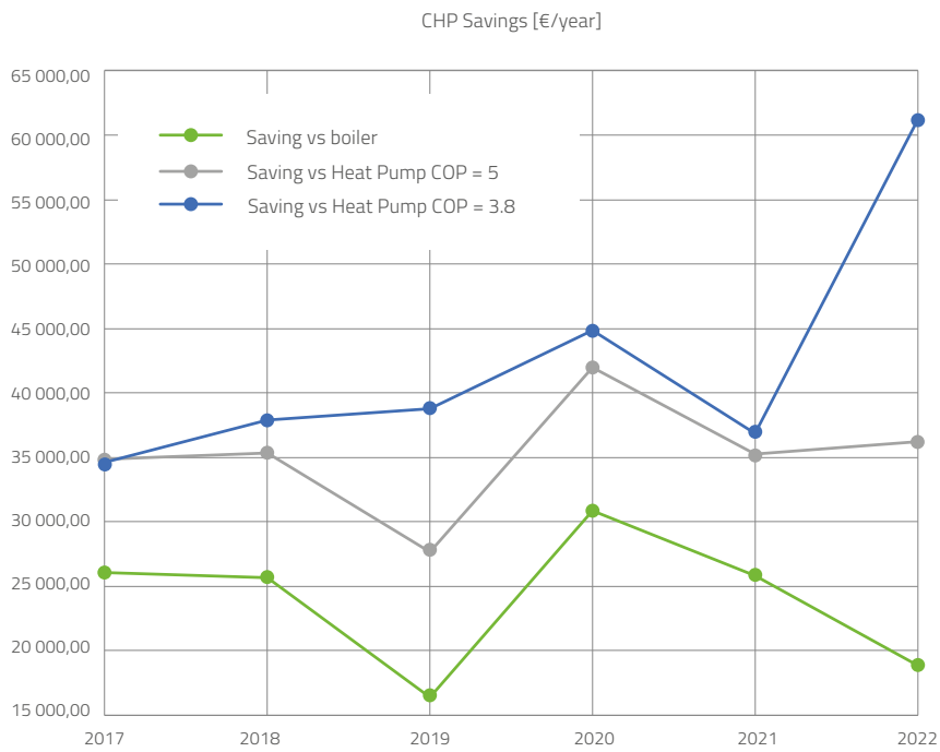
Figure 10: Estimate of annual saving obtained by the hotel operating one 100kW microturbine CHP for 6500 hours
