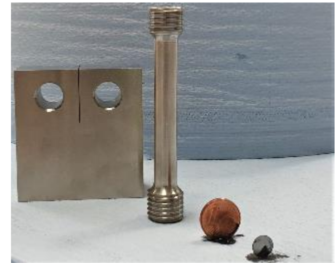
Small punch specimen (right) compared to tensile and CT-specimen
