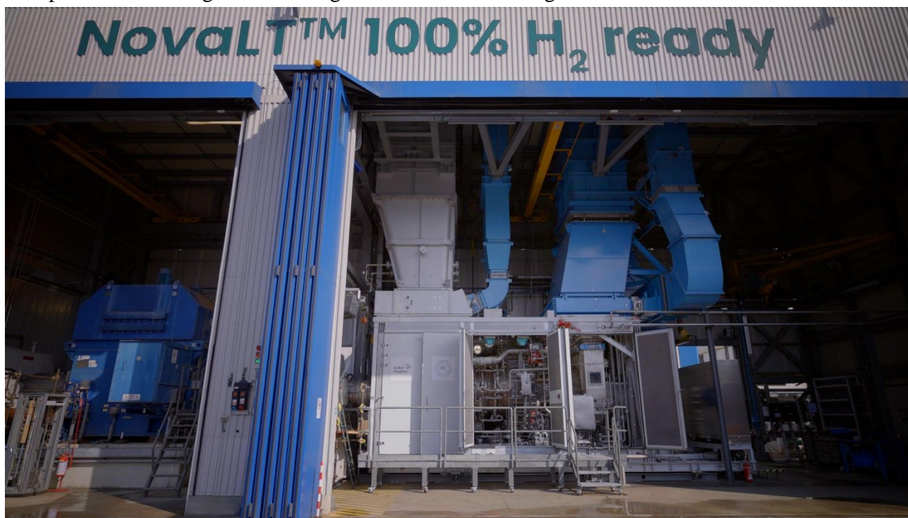
Baker Hughes NovaLT™16 (*) gas turbine, 100% H 2 ready, on dedicated Baker Hughes test bench at Florence (IT).
