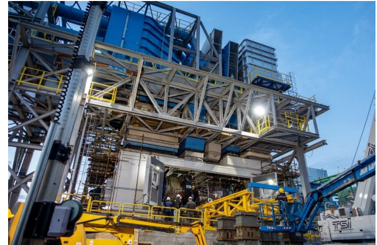
The LM9000 gas turbine was tested at full speed and full load at the Baker Hughes Gas Technology turbomachinery testing facility in Massa, Italy.
