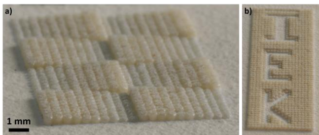
Figure 6: Examples of Clad2Z height variations: (a) 8 areas of dimension 5x5 mm 2 with graded height of 200– 500 µm, (b) cut-outs of shape I-E-K with total area size of 10x30 mm 2 .
