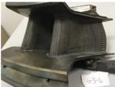
Figure 6 -S1N disassembled after first prototype test
