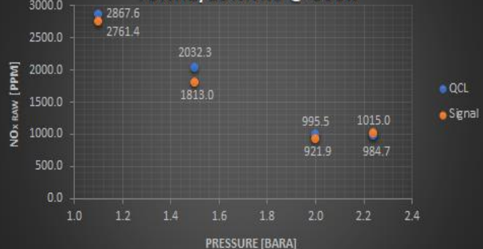
Fully Pre-mixed Swirl Burner. 75%H 2 /25%NH 3 @ 500K
