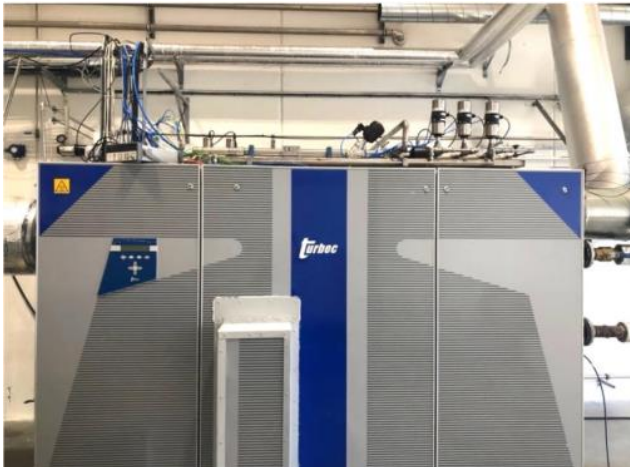
Figure 3: Turbec T100 with F400s.3 Combustor and Modified Fuel Train.
