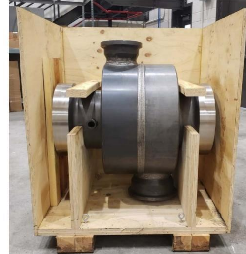
Figure 12 –Turbine Casing – fabricated IN 625
