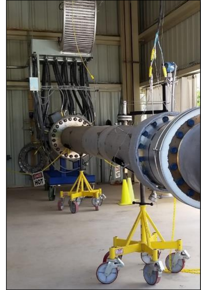
Pre-heated air is supplied to the combustor to mimic typical compressor discharge temperatures
