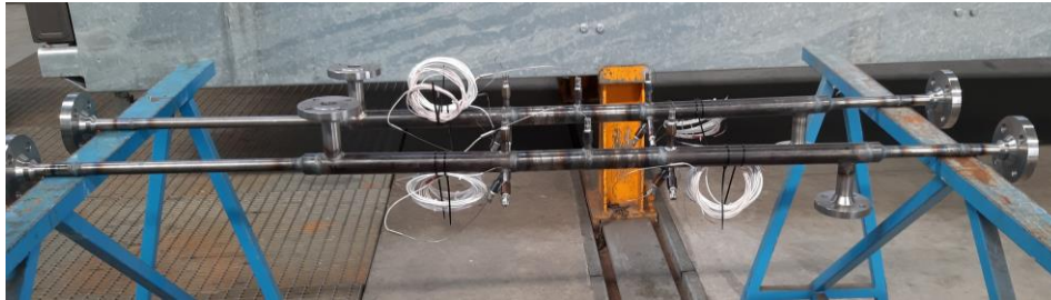
Figure 2: position of the temperature sensors at the cross section of the current test tube.
