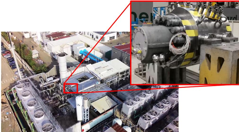
sCO<sub>2</sub> compressor prototype
