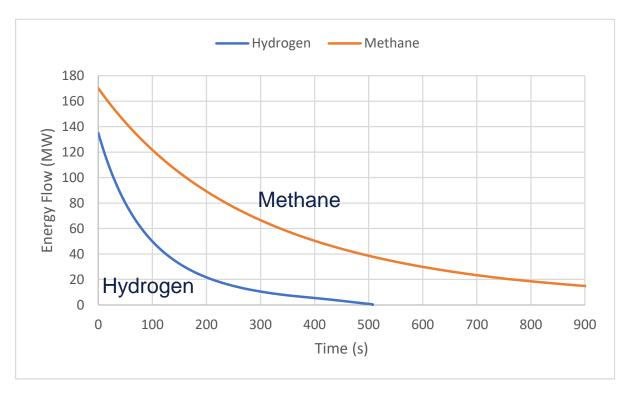
20 mm release from 27 m<sup>3</sup> vessel @70 bar
