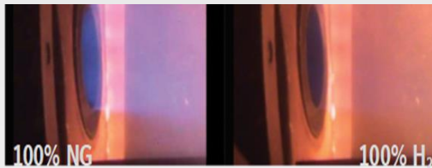
Comparison of Natural gas and Hydrogen flames.
