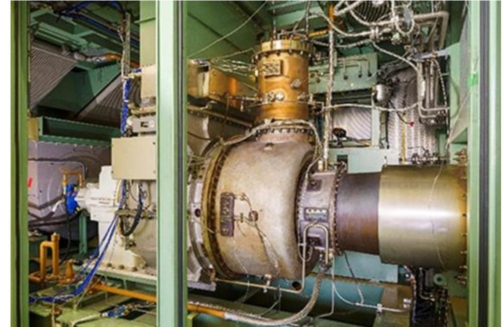
2,000-kilowatt-class gas turbine co-firing liquid ammonia and natural gas at IHI Yokohama Works
