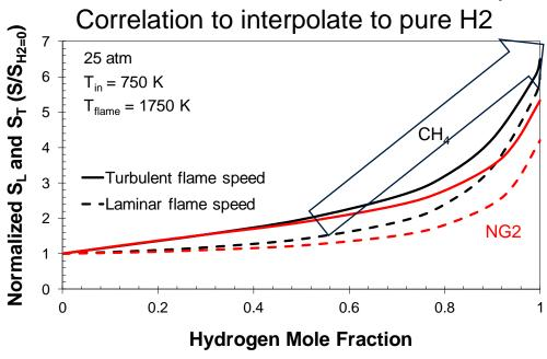
S<sub>T</sub> increases more at lower H<sub>2</sub> content than S<sub>L</sub>
