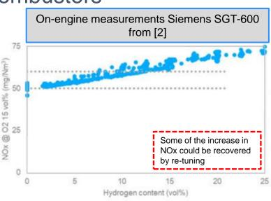
Measurements on current gas turbine combustors indicate a significant increase in NOx as hydrogen is added to natural gas
