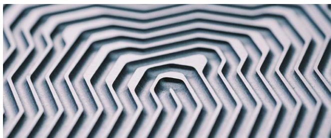
Chemically etched plates used in PCHEs
