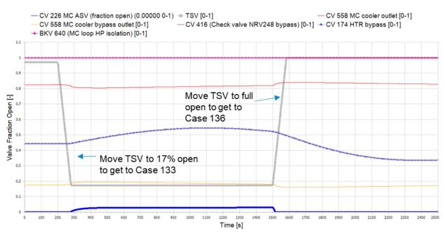
TSV = Turbine Stop Valve ASV = Anti-surge valve MC = Main Compressor
