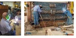
Heater coil operates at 265 bar and 700°C
