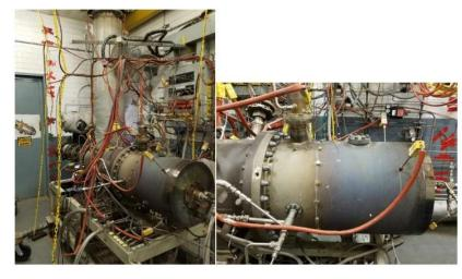
The single injector rig installation located at Solar Turbines combustion test facility.
