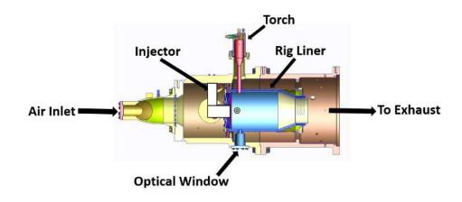
The cross section of the single injector rig
