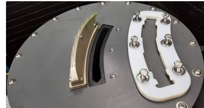
Flow Bench * Gasket and clamp were printed on a PolyJet printer (plastic)
