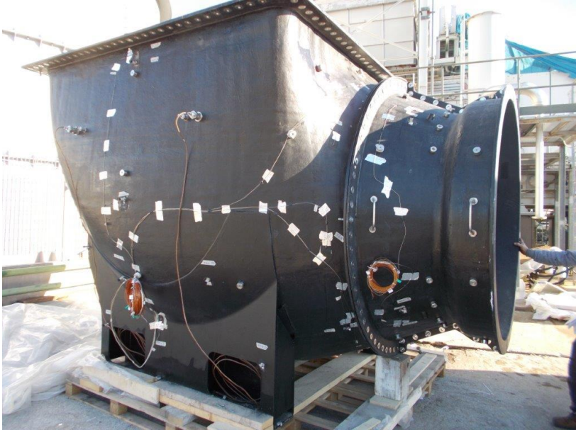
Instrumented and ready for installation
