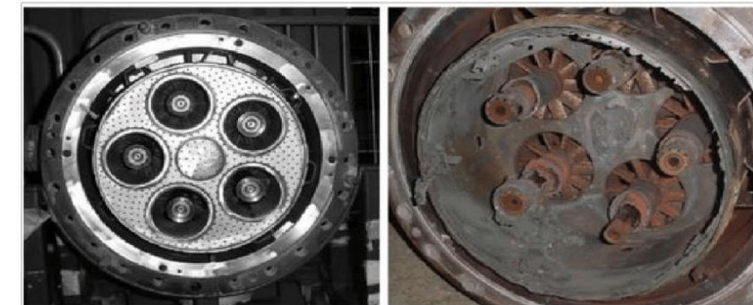
Fig. Damage due to high dynamics
