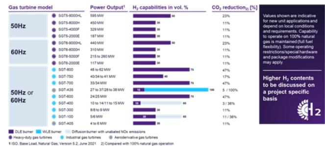
Figure 12: SE gas turbine portfolio hydrogen capability for new unit applications with high hydrogen option
