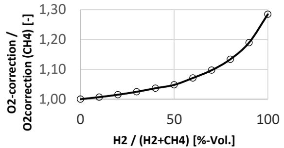
Figure 5: O<sub>2</sub> correction factor
