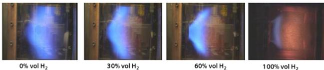
Figure 16: Flame pictures from atmospheric combustion tests in the rig shown above, as H<sub>2</sub> percentage is increased
