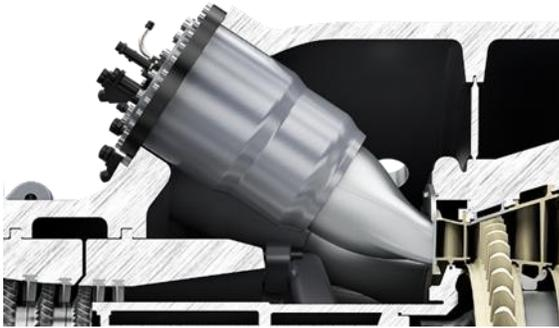
Figure 11: SGT5/6-9000HL combustion system
