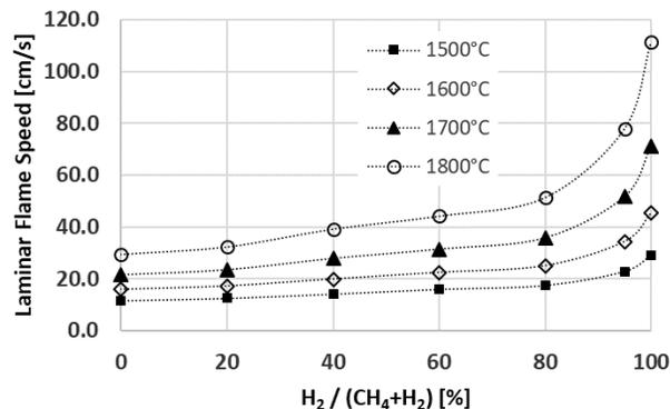
Figure 1: Laminar flame speed of H<sub>2</sub>+CH<sub>4</sub> mixtures under gas turbine relevant conditions
