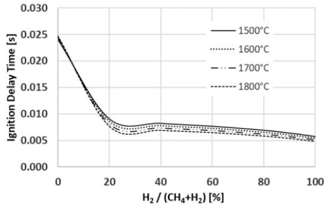
Figure 2: Ignition delay time of H<sub>2</sub>+CH<sub>4</sub> mixtures under gas turbine relevant conditions
