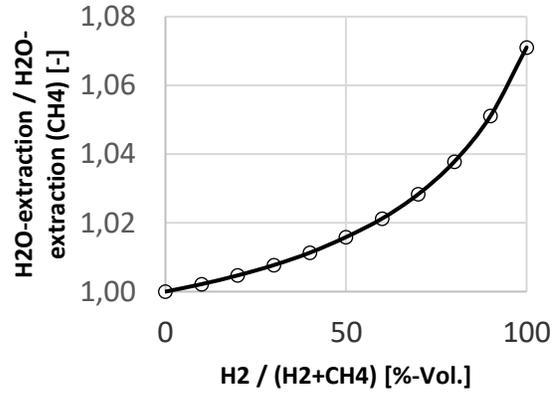
Figure 4: H<sub>2</sub>O extraction factor
