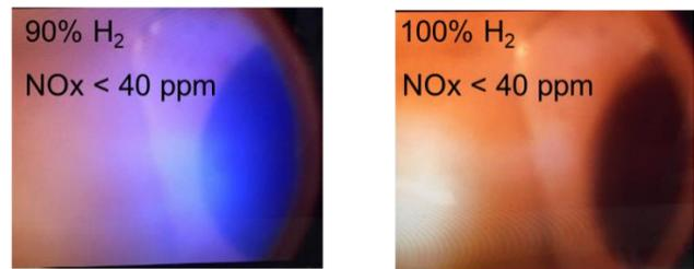
Figure 19: Single-burner high hydrogen test in CEC
