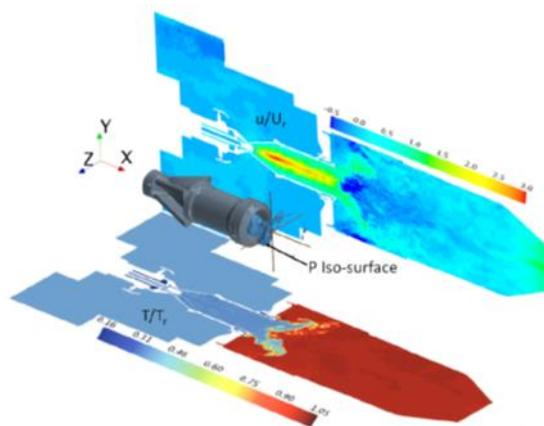
Figure 15: CFD flow field overview from a study of SGT-800 3rd generation burner with high-hydrogen fuels (Moëll, 2018)
