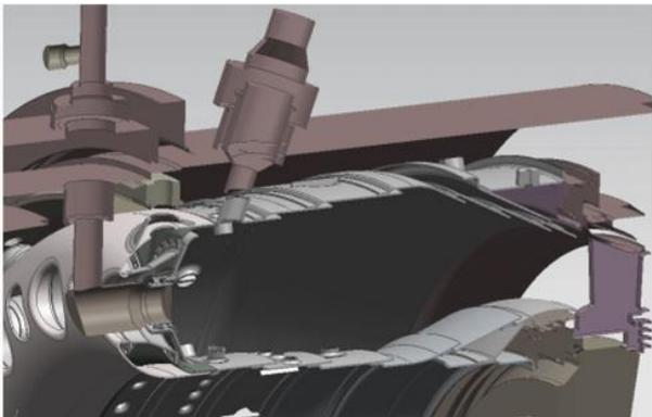
Figure 6: SGT-600 Non-DLE combustion system
