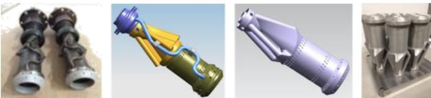
Figure 14: SGT-600, SGT700 and SGT-800 burner design welded with AM repaired burner tip to SLM manufactured still to be cut from printing plate (far right)
