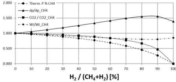
Figure 3: Variation of thermal power from CH<sub>4</sub> and ratio of pressure drop, CO<sub>2</sub> and Wobbe index relative to CH<sub>4</sub> for H<sub>2</sub>+CH<sub>4</sub> mixtures
