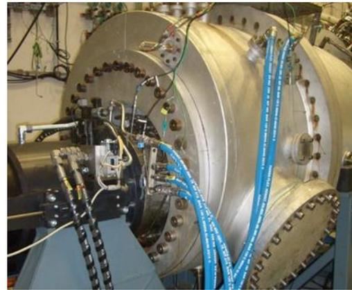
Figure 18: High pressure test rig for combustion tests
