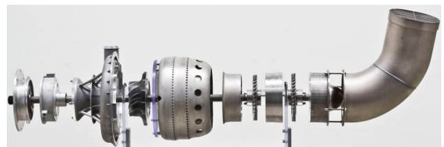
Fig. 2 AM jet engine from Monash University and SAFRAN (Science in Public, 2015).
