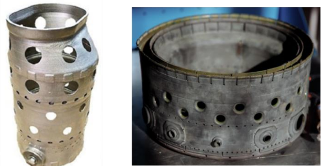
Fig. 8 AM (a) can combustor (Sotov et al., 2019) and (b) annular combustor from Samara University (2018)
