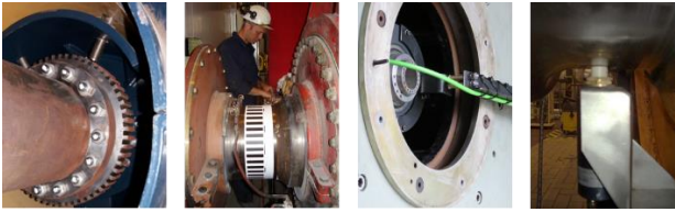
Figure 3: A couple of measurement techniques for torsional vibrations in turbomachinery. From left to right: Hall-effect sensor facing toothed wheel, optical sensor facing zebra-tape, encoder at shaft end, magneto-strictive sensor.
