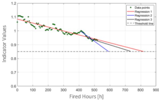
**Figure 1.** Prediction of the RUL with different input data lengths
