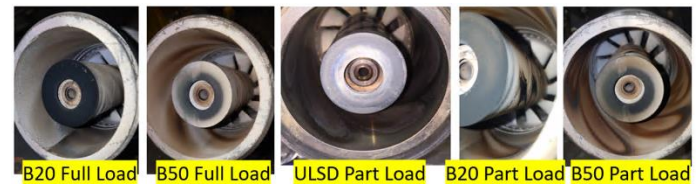
Figure 8. Minimal carbon deposits inside the Titan 130 injector after four hours endurance tests using B20 and B50 fuels at full load and part load conditions compared to ULSD at part load condition
