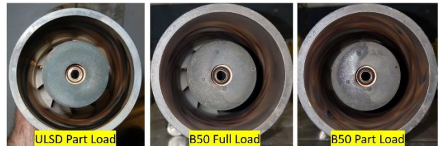
Figure 12 Negligible carbon deposits inside the Taurus 70 injector after four hours endurance tests using B50 fuel at full load and part load conditions.
