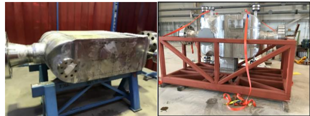
Figure 11 – PCHE type main cooler
