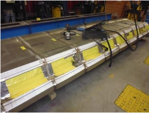
Figure 12 – HTR core assembly (joining of 10 separate PCHE blocks)
