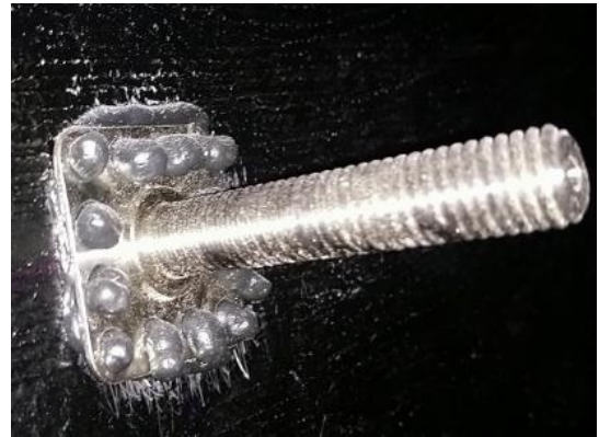
Figure 20. Metal insert bonded to plenum shell
