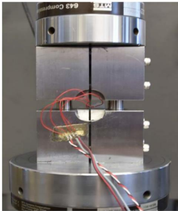
Figure 23. ASTM D6641/D6641M-16e1 compression test
