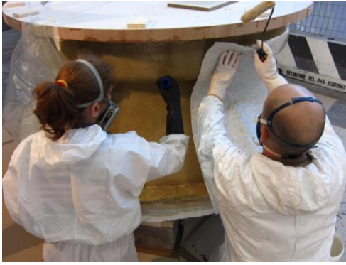
Figure 18. Hand layup of fiberglass
