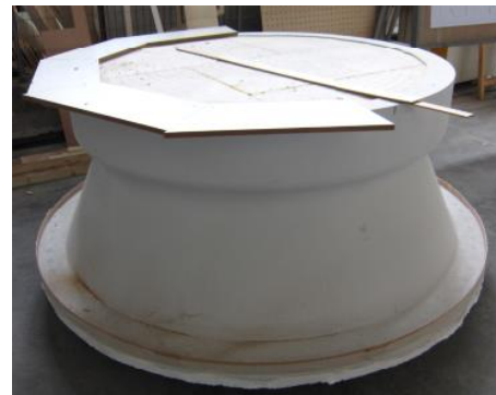
Figure 17. Mold for the composite plenum
