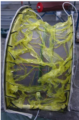
Figure 19. Resin infusion technology
