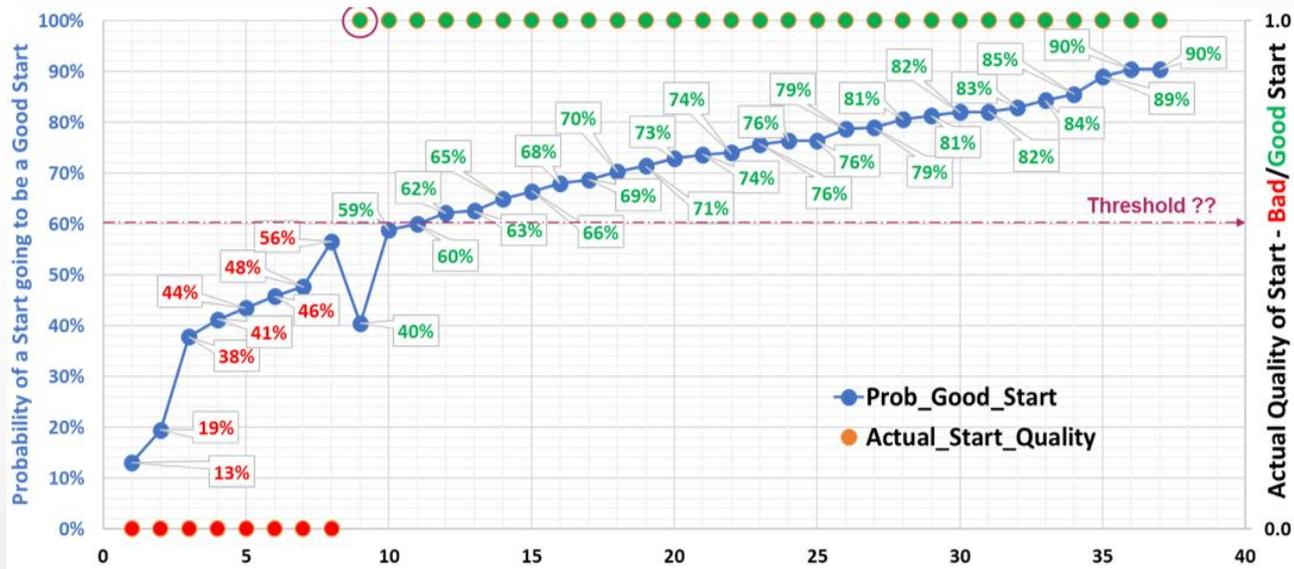
Predictive capability of a trained CNN- Model (Convolutional Neural Network): Probability figures show the ratio of true vs. false predictions for each difference image
