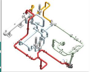
Test arrangement to sCO<sub>2</sub> CC prototype
