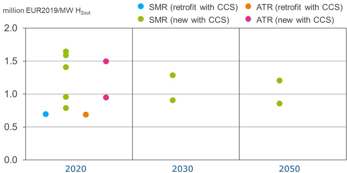
Figure 2-2: Investment cost for blue hydrogen production technologies
