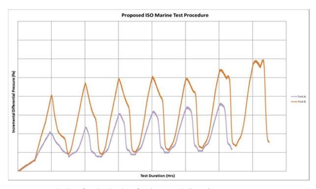
Constant loading of NaCl and cycling of RH (no water challenges)
