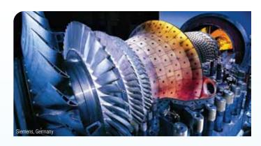
**COMBUSTION** (SP1) – Safe and low emission combustion technology for undiluted, hydrogen-rich syngas will be developed and demonstrated. In order to achieve this, problems resulting from the differences in combustion properties of hydrogen and natural gas need to be addressed and solved. These are higher flame speed, higher adiabatic flame temperature, drastically reduced auto-ignition delay times and the large increase in volumetric fuel flow rate of hydrogen compared to natural gas.
