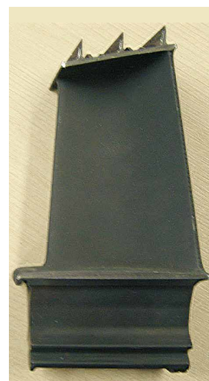
Figure 10: Image of Siemens V64.3 gas turbine blade being used for coating demonstration trials in the EC FP7 H 2 -IGCC Project
