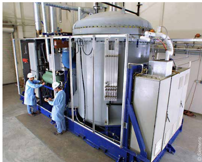
Figure 6: Picture of a Solid Oxide Fuel Cell/Gas Turbine hybrid system
