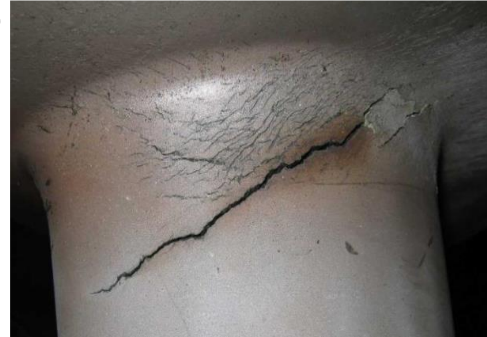
Cracks on 2nd stage nozzle of F-class gas turbine (Source: EDF, Jean Luis Meyer , EXPECTATIONS OF AN OPERATOR ON GT COMPONENTS LIFE ASSESSMENT)
