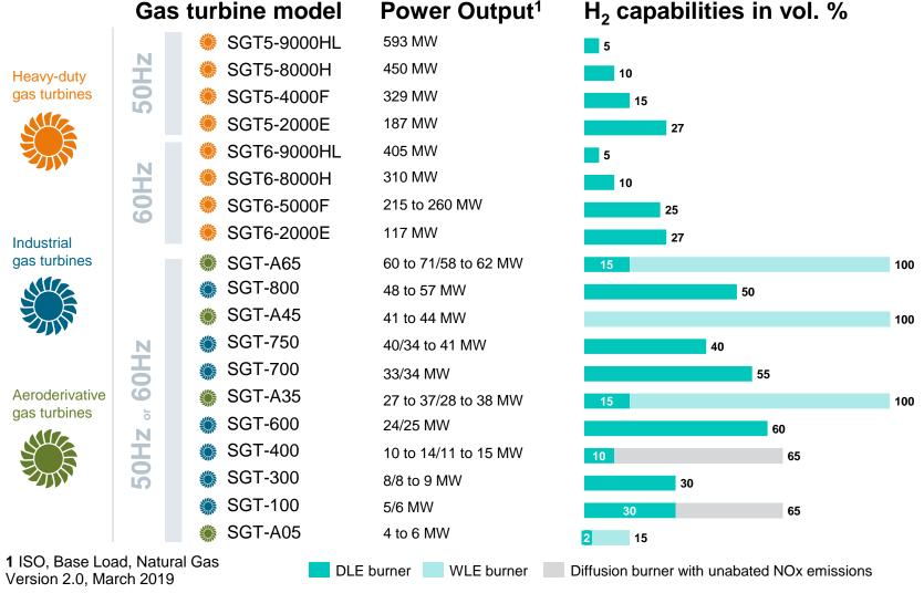
Values shown are indicative for new unit applications and depend on local conditions and requirements. Some operating restrictions/special hardware and package modifications may apply. Any project >25% requires dedicated engineering for package certification.
